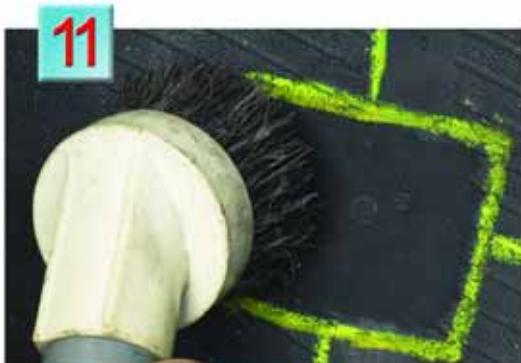
**11.** Use a vacuum to remove the buffering dust.
