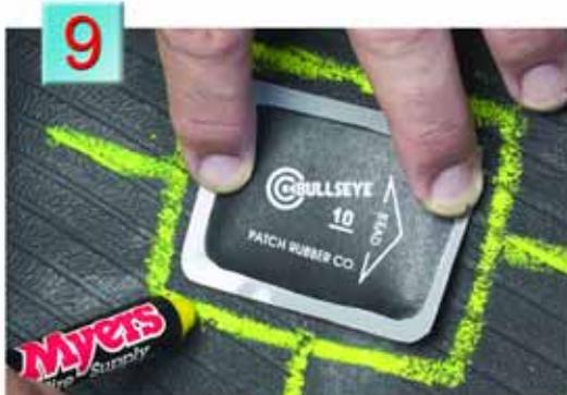
**9.** Making sure the bead arrows of the repair unit are pointing to the beads, center the repair unit over the injury. Use a tire crayon and outline an area 1/2" larger than the repair unit.
