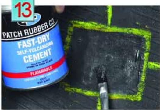
**13.** Apply an even coat of Patch Rubber Fast-Dry Self-Vulcanizing Cement to the entire buffed area. Allow cement to dry until tacky. Never use blow dryers, compressed air, or heat lamps to facilitate drying. Drying time is affected by temperature and humidity.
