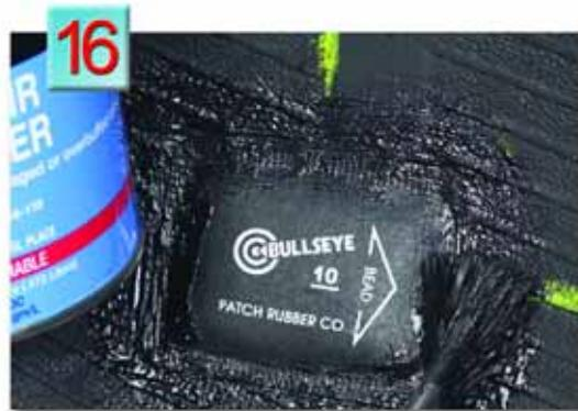
**16.** Apply Patch Rubber Repair Sealer to the overbuff area.
