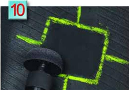
**10.** Use a low speed buffer (max. 5,000 RPM) and a buffering rasp to buff the plug and the outlined innerliner area. (RMA #1 Buffing Texture). BE CAREFUL NOT TO BUFF THROUGH THE INNERLINER.
