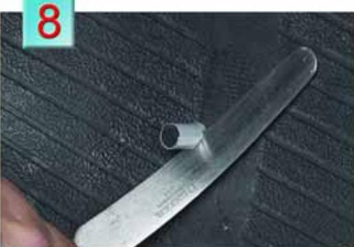
**8.** Using a flexible knife, cut the plug on the inside of the tire 1/8" above the innerliner. Be careful not to stretch the plug when cutting.
