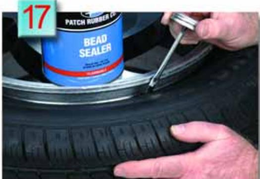
**17.** Apply Patch Rubber Bead Sealer to the bead of the tire before inflation to help prevent air loss around the bead.
