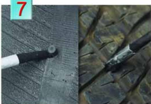
**7.** While the cement is still wet, push the wire puller through the injury from the inside of the tire. Grasping the wire, use a steady pull until 1/2" of the gray rubber on the plug is exposed outside the tire.
