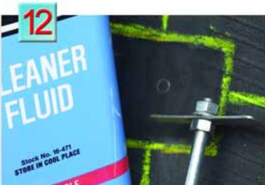
**12.** Apply a light coat of Patch Rubber Cleaner Fluid to the buffed area, scrape clean and allow to dry.
