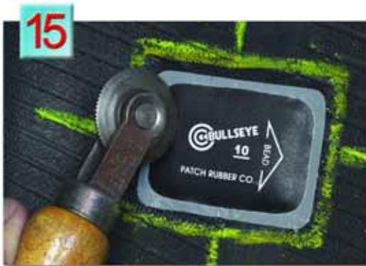
**15.** Stitch the repair unit vigorously from the center working outwardly. Use as much hand pressure as possible. Remove top cover film.
