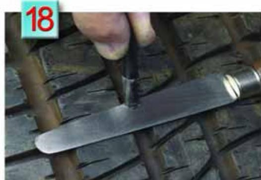
**18.** After inflating, cut the plug flush with the outside tread area. Return tire to service.
